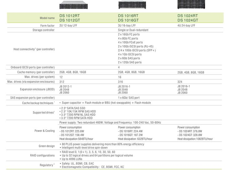
$<sup>1. \,</sup> Eon Stor \, DS \, 1000G \, models: \, super \, capacitor \, and \, flash \, module \, or \, BBU \, + \, flash \, module \, optional \, and \, not \, included \, by \, default.$
